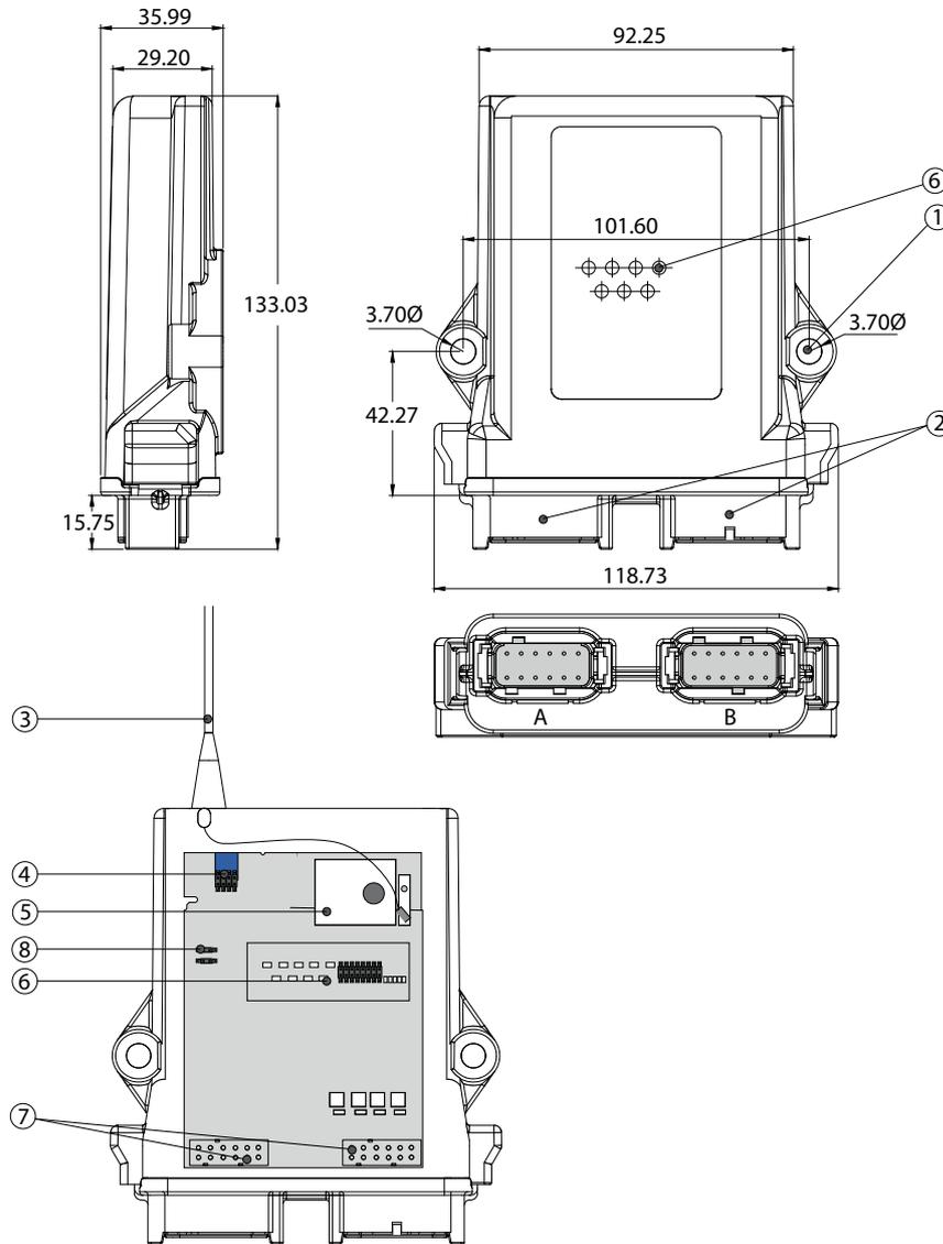
1. Fixing slots (fixed assembly or anti-vibration)
