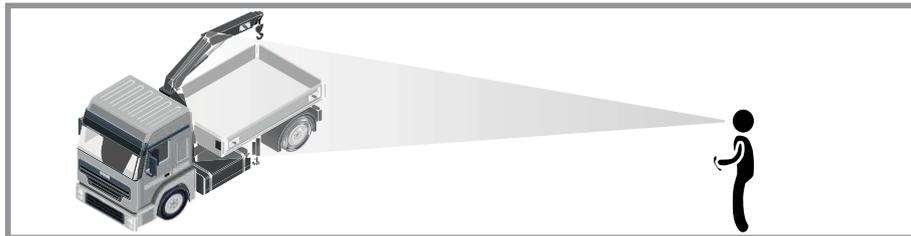
2. Optional: If it is difficult to achieve direct vision between the receiver's antenna and the transmitter's working area, it is recommended to use an extended antenna in a clear location (only for models that allow an antenna).
