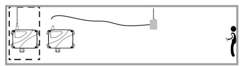
**3.** Proceed to connect the power supply. Use the connection block diagram provided with the system, where the correspondence between the transmitter maneuvers and the receiver's outputs are detailed.
